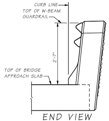
W-BEAM SHOWN WITH "D" CONNECTION OR "F" CONNECTION (SEE STD. PLAN C-5).
