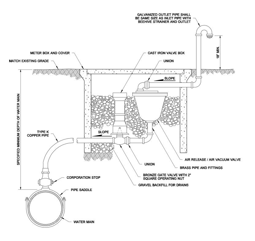
1. The size of the combination air release / air vacuum valve shall be specified in the Contract. The piping and valves shall be the same size as the combination air release / air vacuum valve.
