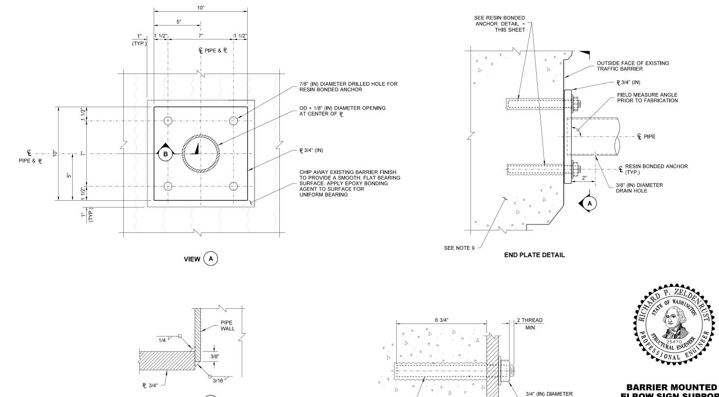
3/4" (IN) DIAMETER RESIN BONDED ANCHOR
