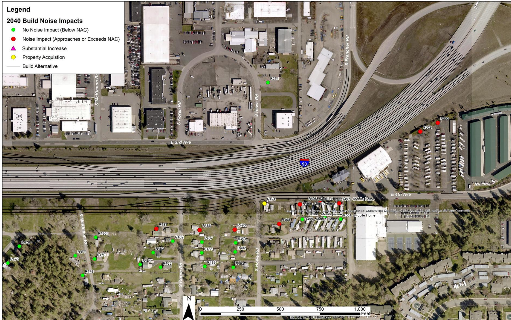
Exhibit 21: Modeled 2040 Build Noise Abatement Criteria Impacts – Project Area East Terminus at I-90/Sprague Avenue
