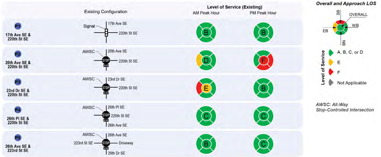
Exhibit 4-4. Existing Intersection Analysis Results, Sheet 3 of 3
