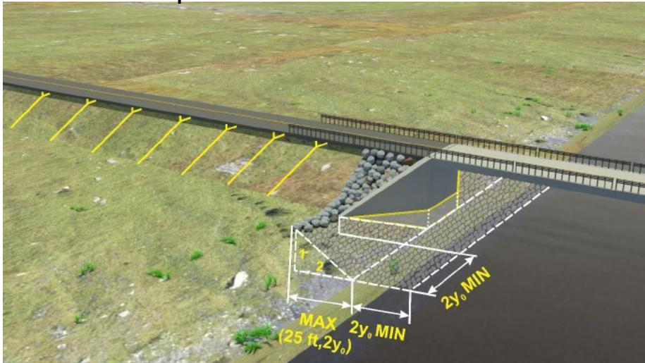
**Scour Condition B** uses overbank channel hydraulic values to compute abutment scour depths.
